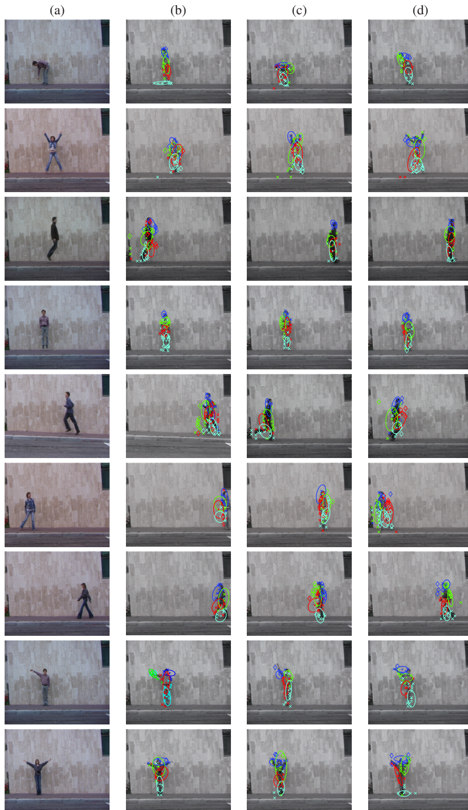
Figure 10. Learnt action models: Each row illustrate a different action category: bend, jack, jump, p-jump, run, side, walk, wave1, wave2. Column (a) shows example frames from the original sequence. (b)-(d) show the three mixture components for each action model. Static features are represented by crosses and motion features by diamonds. Each image feature is colored according to its part membership. Ellipses illustrate the variance of the position distributions for each part. The figure is best viewed in color.
